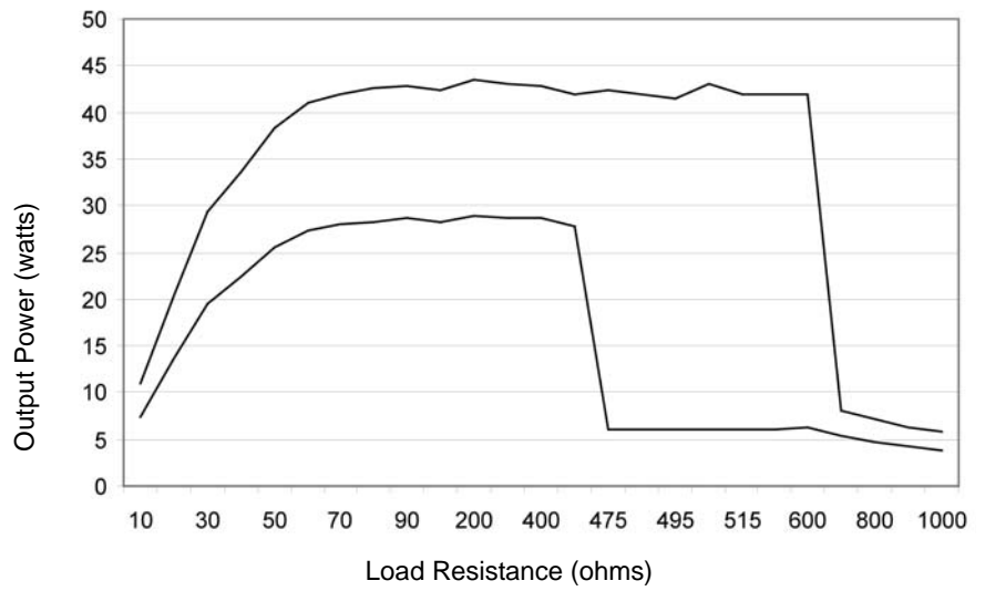
Output power vs. impedance for Standard bipolar 35W mode
