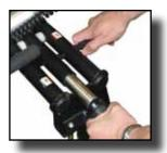
**1.** While holding onto the Swivel Release Knob, pull out the T Handle.
