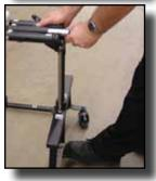
**5.** Step on the Height Adjustment Pedal and pull up on the Clamp Support Assembly to raise the unit. When necessary, step on the Height Adjustment Pedal while pressing down on the unit to lower the unit.
