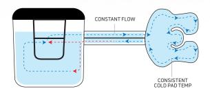
**ICEMAN** with dual pump recirculation technology. The DonJoy® IceMan® features a patented recirculation system that allows water warmed after flowing through the cold pad to be preserved and remixed with cooler ice water at a constant flow rate, providing consistent cool water distribution throughout the cold pad.
