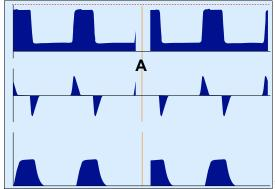
The current curves are immediately frozen. The cursor (A) displays the time of "freezing" and the value at the cursor position.
