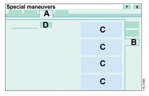
Evita V300 displays the NIF values of the last measurements, including the time and date (C).
