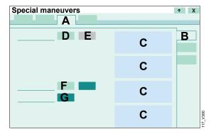
Evita V300 displays the P0.1 values of the 4 previous measurements (C).
