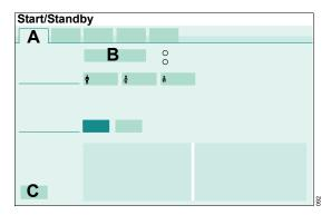
**2** Touch the *Start ventilation* button (B) and confirm with the rotary knob.
