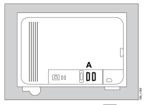
Connect an external device to the OO COM 1 or the COM 2 (A) interface of Infinity C300.
