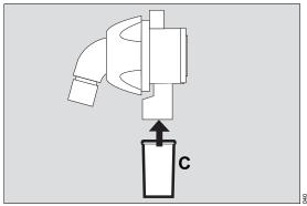
**3** Fit the water trap container (C).
