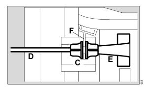
3 Clip the protective sleeve (C) immediately after the connector (E) onto the system cable (D). Align the protective sleeve so that the slots of the protective sleeve are facing downwards and upwards.
