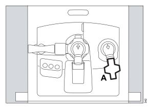
Fit the bacterial filter (A) onto the inspiratory port.
