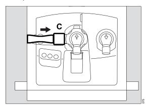
3 Push the flow sensor to the right up to the stop in the flow sensor sleeve (C) of the Infinity ID expiratory valve.
