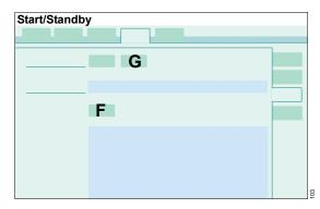
5 If the displayed leakage value is permanently below 120 mL/min, the OK button (F) turns light green.
