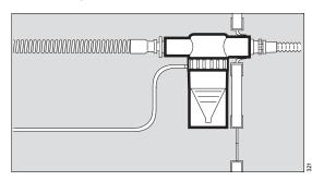
Push the inlet port or the outlet port of the medication nebulizer into the upper hose guide of the incubator.
