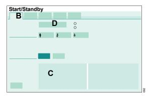
Evita V300 displays the ventilation parameter startup settings (C). The **Start ventilation** button (D) can be used to start the therapy. When the therapy is started, the settings become effective.
