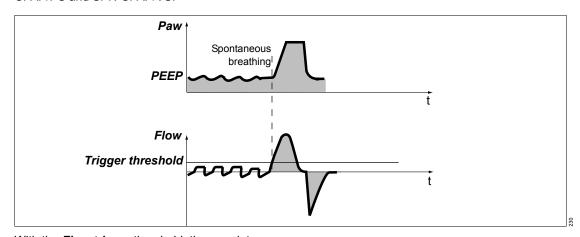
With the *Flow trigger* threshold, the mandatory breaths are synchronized with the inspiratory efforts. The start setting of the flow trigger can be configured on the page *System setup* > *Ventilation* > *Start settings* > *VT, RR, Trigger* page.
