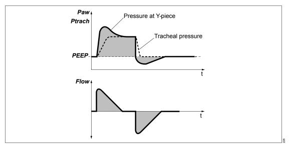
**ATC** regulates the airway pressure to the tracheal level. This function calculates and displays the tracheal pressure on the basis of a mathematical tube model, the set tube type and the inner diameter of the tube.
