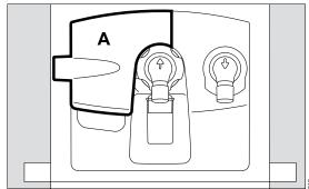
1 Open the flap (A) by lifting the lower edge upwards.
