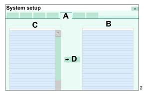
Evita V300 displays the already installed applications (B) and the applications available on the SIM card (C).
