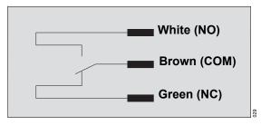
As soon as Evita V300 signals an alarm, the connection between the white cable and the brown cable (NO and COM) is closed and the nurse call is activated.
