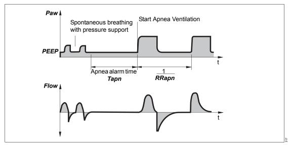
For Evita V300 to be able to detect an apnea, flow measurement with the neonatal flow sensor must function and flow monitoring with the neonatal flow sensor must be activated.
