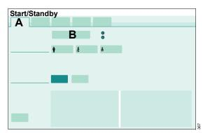
2 Touch the *Start ventilation* button (B) and confirm with the rotary knob.
