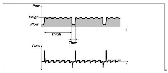
The patient breathes spontaneously at a high pressure level *Phigh* for an adjustable length of time *Thigh*. For very short expiratory times *Tlow*, Evita V300 switches to a low pressure level *Plow*. The normal lung areas are emptied, but the "slow" lung areas only change volume to a lesser extent\*.
