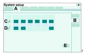
Evita V300 displays the start-up values used for the alarm limits.
