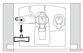
3 Remove the flow sensor from the socket (C).
