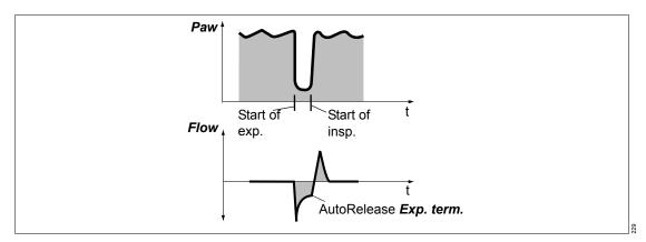
In ventilation mode PC-APRV, the duration of pressure release is determined from the expiratory flow curve when *AutoRelease* is activated. The *Exp. term.* setting specifies when the ventilation returns to the pressure level *Phigh* dependent on the decline in percent of the peak expiratory flow. The *Tlow max* therapy control limits the maximum duration of pressure release.
