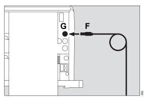
5 Insert the connector (F) of the flow sensor cable into the socket (G) at the rear of Evita V300.
