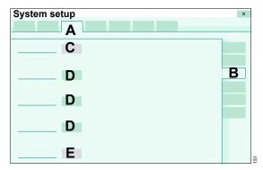
Evita V300 displays the start mode (C) and 3 ventilation modes (D). These ventilation modes are displayed in the *Ventilation settings* dialog window after Evita V300 has been started.
