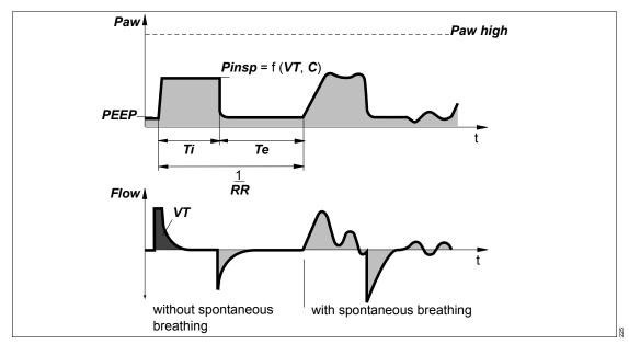
Evita V300 provides ventilation with AutoFlow/Volume Guarantee with a decreasing flow in order to avoid pressure peaks. Evita V300 determines the pressure required for the set tidal volume, with consideration of the lung conditions (compliance, resistance) and the patient's spontaneous breathing demand.
