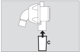
4 Fit the water trap container (C).
