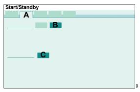
4 Touch the NIV button (B) and confirm with the rotary knob.
