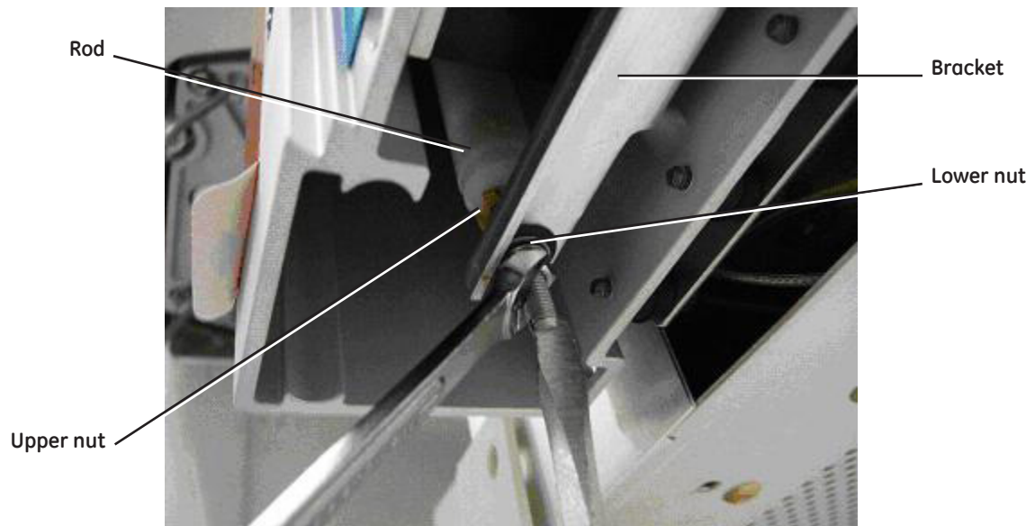
Figure 5-46 Removal of the Lower M5 Nut
