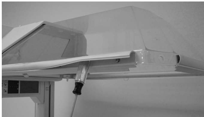
Figure 5-8 Wedging a Blunt Object to Keep Seal Open
