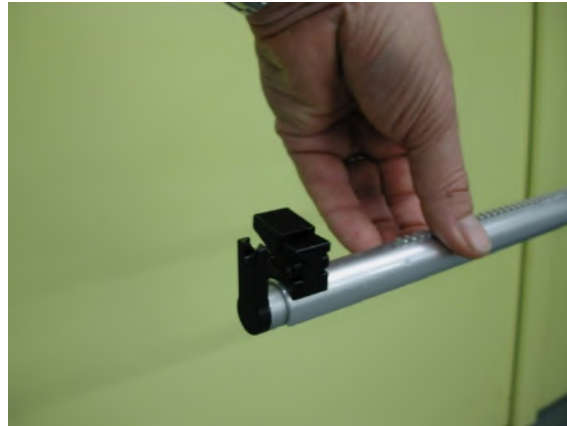
Figure 5: Mobile clamp moving toward catheter guide
