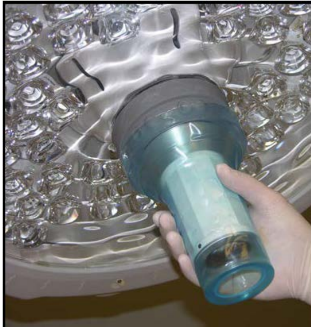
Figure 5-11. Install Disposable Sterile Camera Cover
