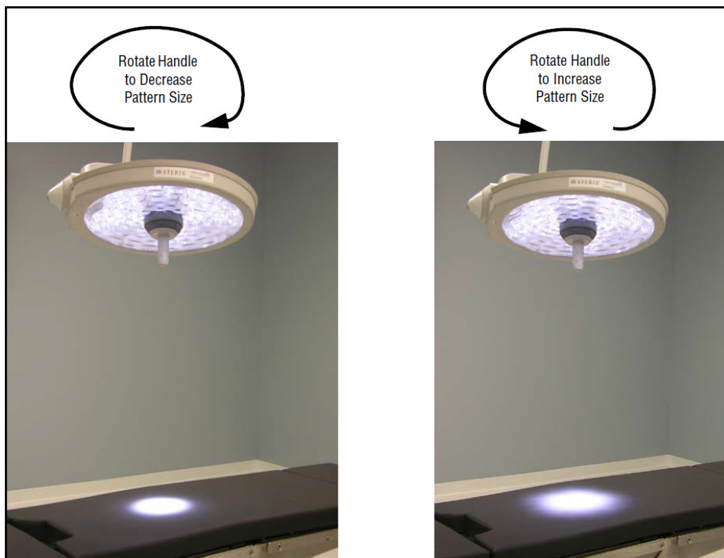
Figure 5-5. G5 Lighthead Pattern Adjustment
